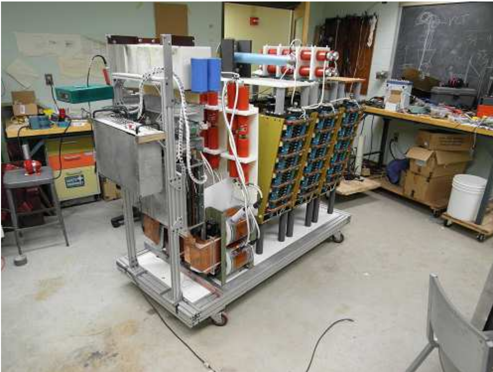
Figure 3.2 Resonant power supply in construction.
