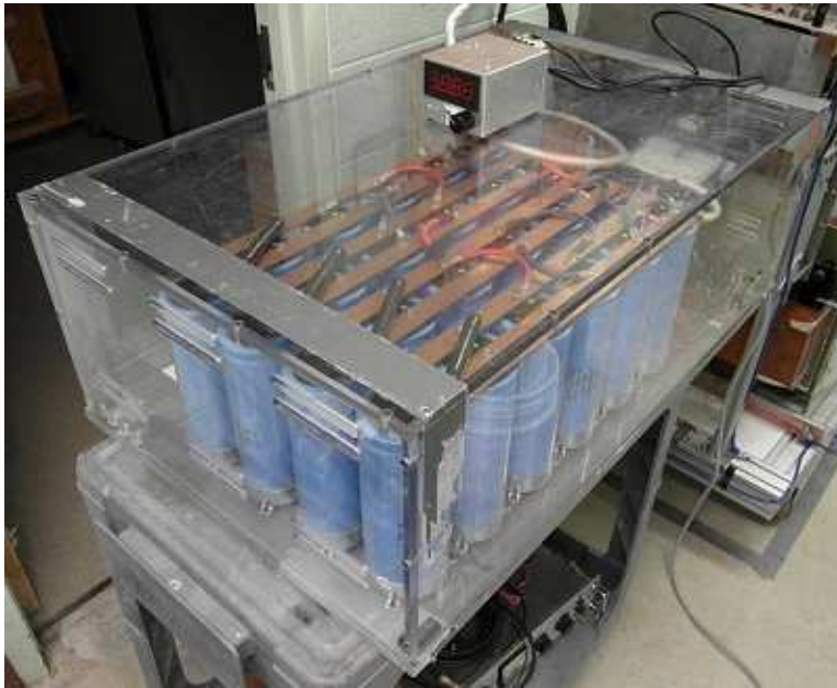
Figure 3.4 Testing capacitor bank.
