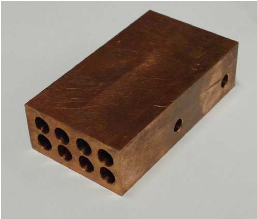
Figure 3.12 Main capacitor bank interconnect block.
